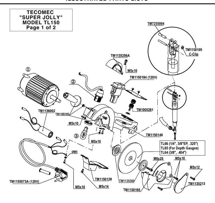
Motor only, 120v — No. TM113614 Motor with arm assembly — No. TM1150163
