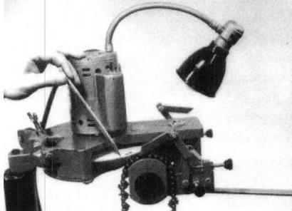
12) Begin sharpening the first tooth, ALWAYS grinding into the tooth. Grind a little at a time, to be sure you don't burn the tooth.
